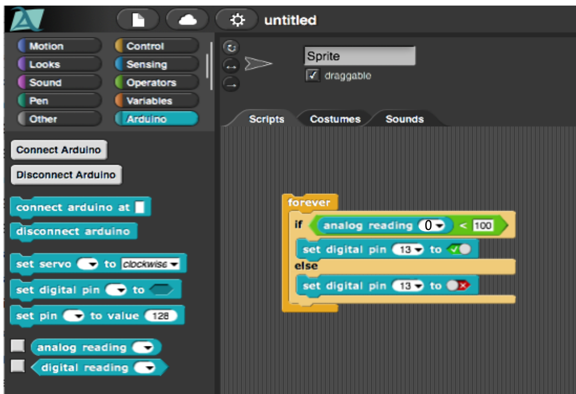
Figure 14. Snap4Arduino connection to Arduino board
