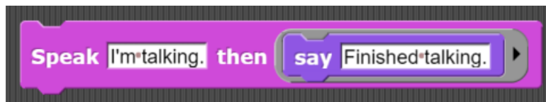
Figure 2 - Simple speak command takes a text argument and an optional continuation function
