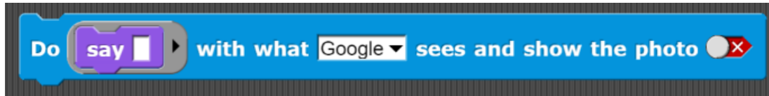
Figure 8 - A simple block for obtaining a list of labels of what is in front of the camera
