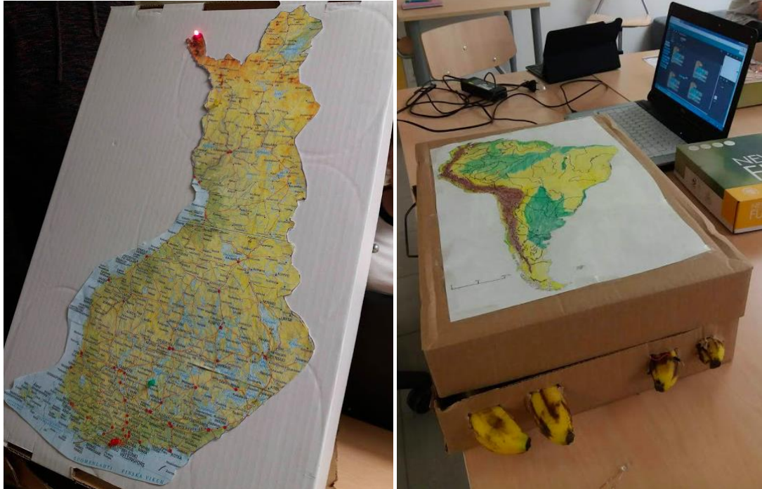
Figure 63: Examples of student projects: LEDs to indicate relevant information on the map when a specific word or question is told or a sensor (banana) is touched
