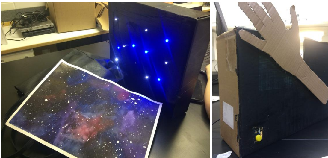
Figure 66: Examples of interactive art projects: a sky with stars (LEDs blinking when touch sensor pressed) and a high-five arm (arm moving with servo motor when button pressed)
