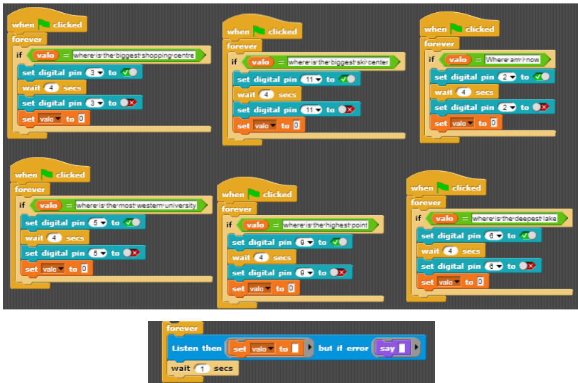
Figure 64: A program code of a map project where and LED lights up to show for example the location of the deepest lake on the map
